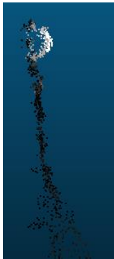
Figure 3: Tripod (black points) with reflective band at the top (white/gray points), measured with the Livox Mid-70 sensor. The reflective band is tightly attached to the cylinder, but the data points are farther away from the tripod axis, due to the highly reflective surface. The distance is about 60 mm from where it should be.
