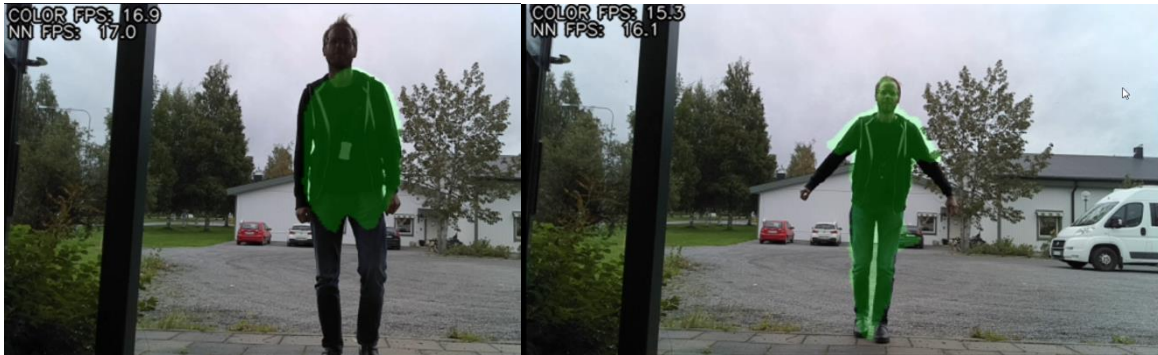
Figure 10: The deeplab_v3p_person module is used to mark the people in the images with the green colored blob, where the pixels of the images are marked where the person is detected, which can be used to extract depth pixel values at the objects, excluding points that do not include the person. The camera used is the OAK-D-Lite camera.
