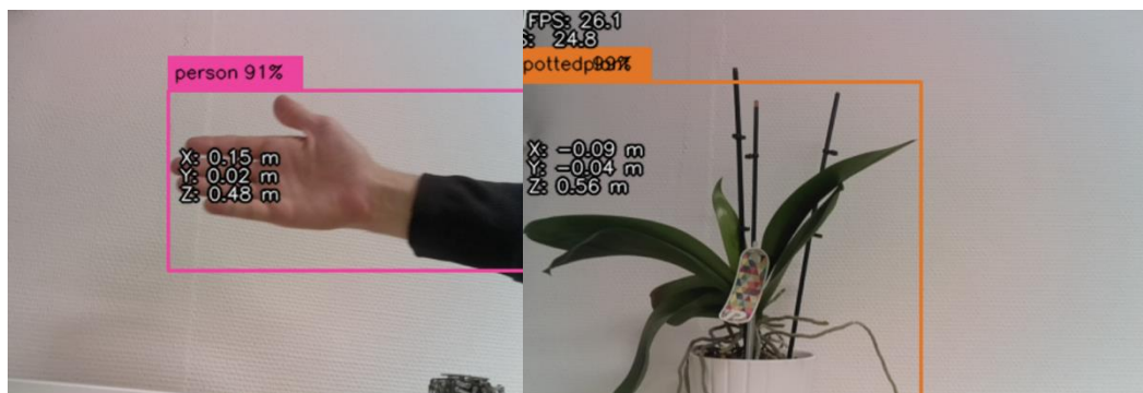
Figure 4: Showing (part of) frames from the OAK-D-Lite camera using the mobilenet-ssd CNN model, identifying certain objects. Left – Hand (of a person) is classified as a person. Right – A potted plant is classified as just that.
