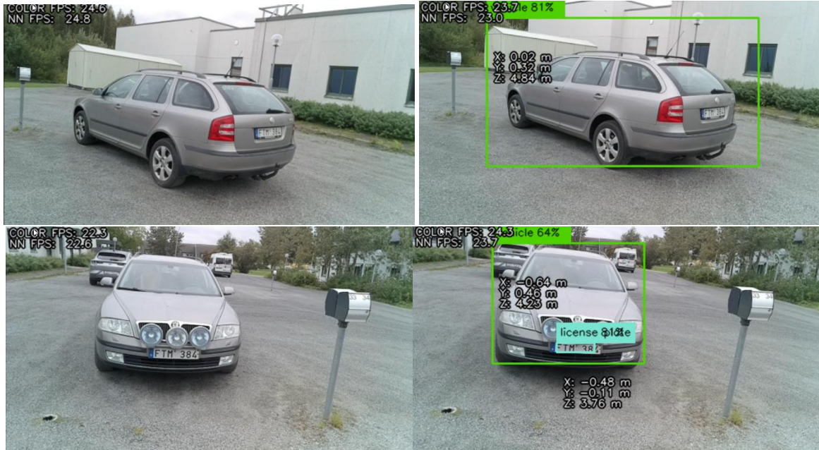
Figure 13: The vehicle_license_plate_detection_barrier working on four different images from the OAK-D-Lite camera. The top two consecutive images from the same stream where the vehicle is not detected in one frame and then detected in the next. Unlike other vehicle detection algorithms, the detection was not very reliable, and the results often jumped back and forth even with images so close in view to each other as those two. The lower two show the same thing but for the license plate detection as well. The model often failed to detect the license plate and could often lose the object between frames.
