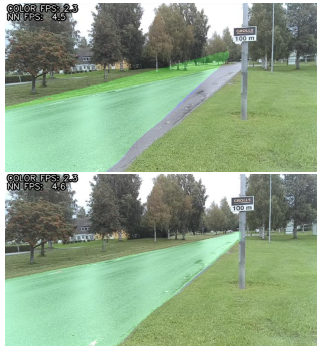
Figure 14: The road_segmentation_adas AI model detecting an asphalt road and visualizing a green layer at the position and shape of the road. The two images show that it takes some frames for the road position to be updated. While holding the OAK-D-Lite camera in a static position the green layer will shape and cover the road, showing that the position of the road is detected.
