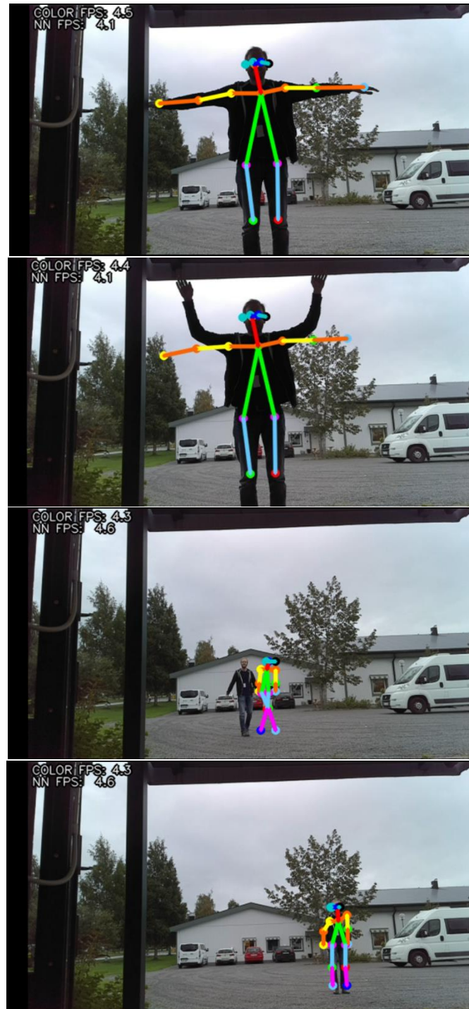
Figure 9: The CNN model human-pose-estimation used for detecting the positions of the human “skeleton”, from 2 m up to about 10 m. The process is intensive for the camera’s processing unit, and the skeleton positions have a hard time keeping up with the camera stream it uses to extract the skeleton position at higher frame rates (> 5 fps here), for the OAK-D-Lite camera.
