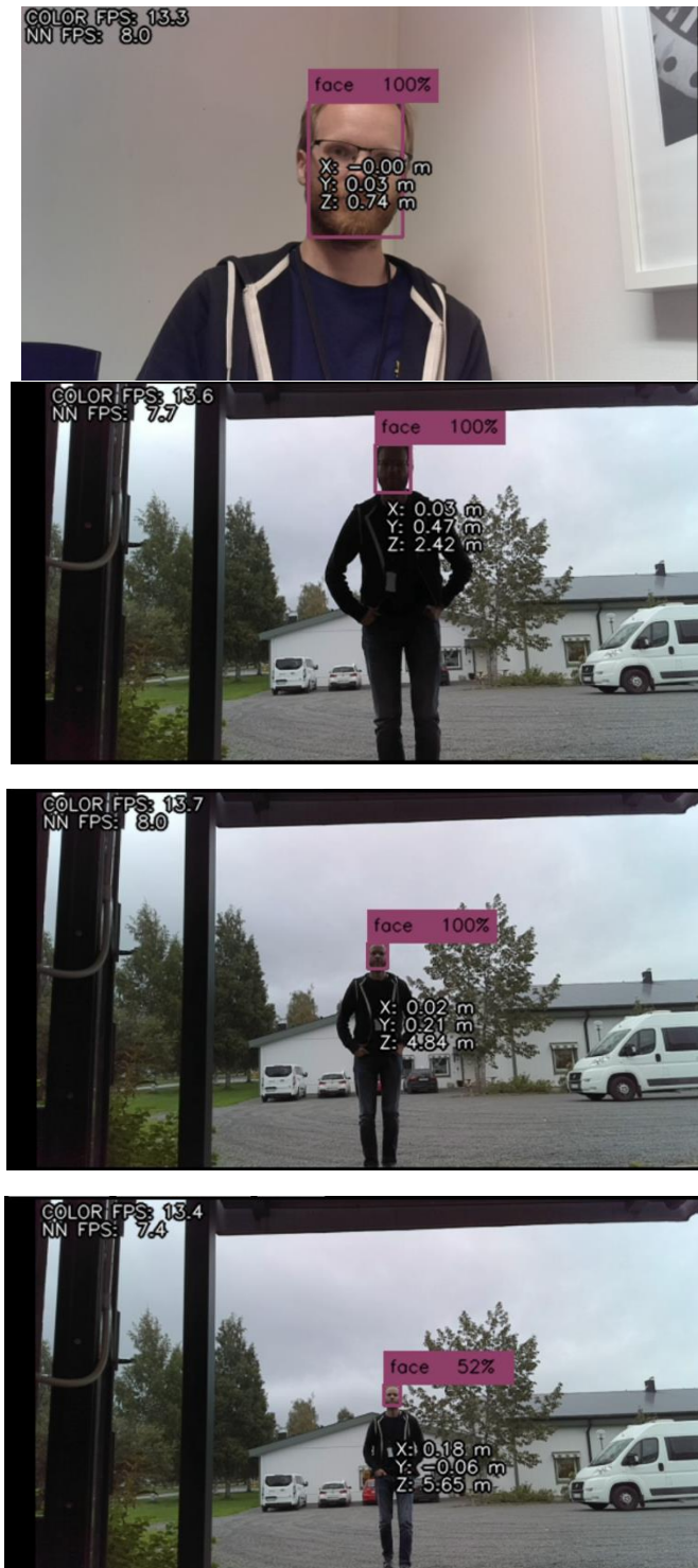
Figure 8: The CNN model face-detections-adas used for detecting humans faces, from 0.7 m up to about 5 m, before losing track of the detected face. The camera used is the OAK-D-Lite camera.
